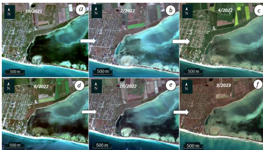
Fig. 3. Chronology of evolutionary stages, showing open (a,c) and closed channel (b,d,e,f) during the period of 2021-2023. Arrows show channel orientation and closed channel (round-end symbol; image source: Land Viewer)
