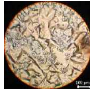
Fig. 6. Image of the surface of a silicon wafer after metal-stimulated etching with d_C=35-40 nm.
