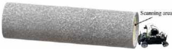
Fig. 1. Example of visualization of the work of the system for finding defects in pipelines using JetRacer Kit
