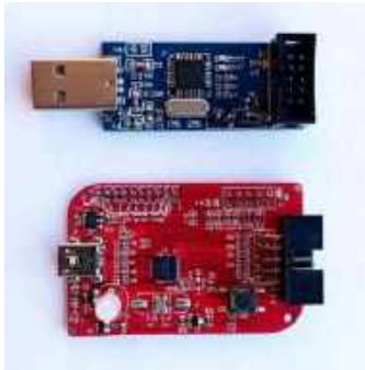
Fig. 3. Various designs of TI CC-Debugger replica (above) and original design (below).
