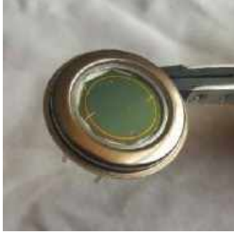
Fig. 1. Silicon four-element p - i - n PD with a guard ring
