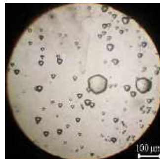
Fig. 5. Surface of a silicon wafer after selective etching for 15 minutes.
