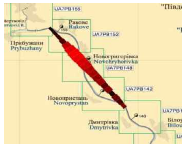
Fig. 11 Change of the speed of the river current in the channel with a variable angle of inclination of the middle line of the bottom.
