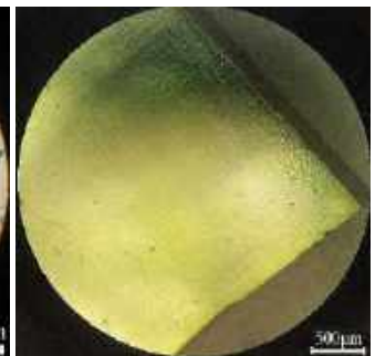
Fig. 6. Surface of a silicon wafer of orientation [100] doped with phosphorus after selective etching.
