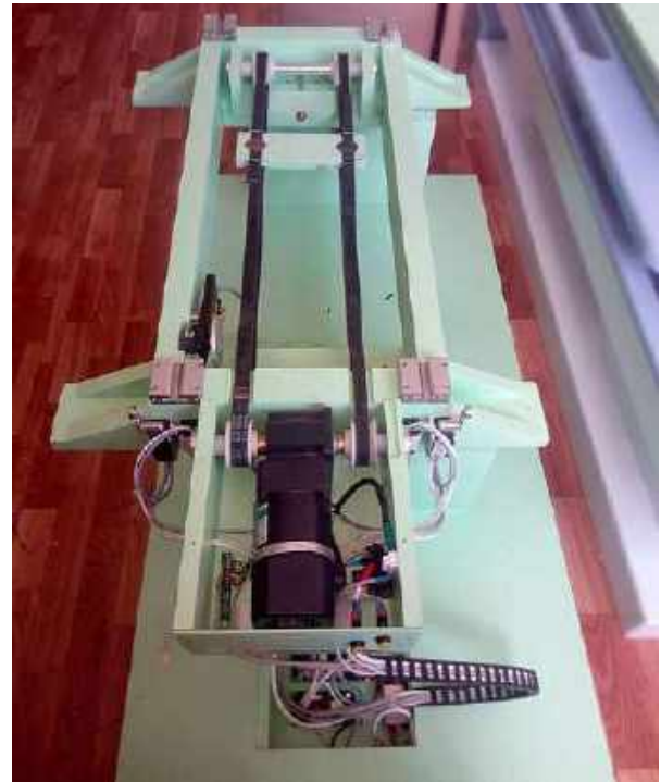
Fig. 10. Design of moving patient's bed (without top platform)
