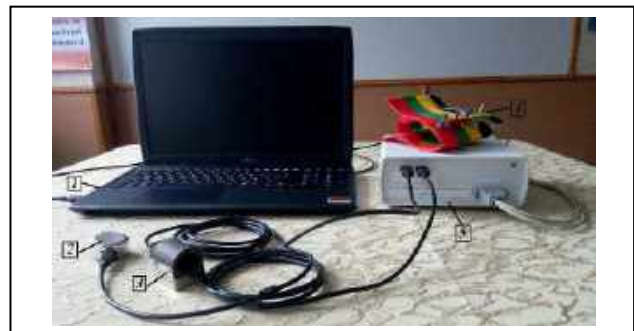
Fig. 1. General view of the complex: 1- laptop; 2, 3 - optical heads; 4 - ECG electrodes; 5 - signal processing unit
